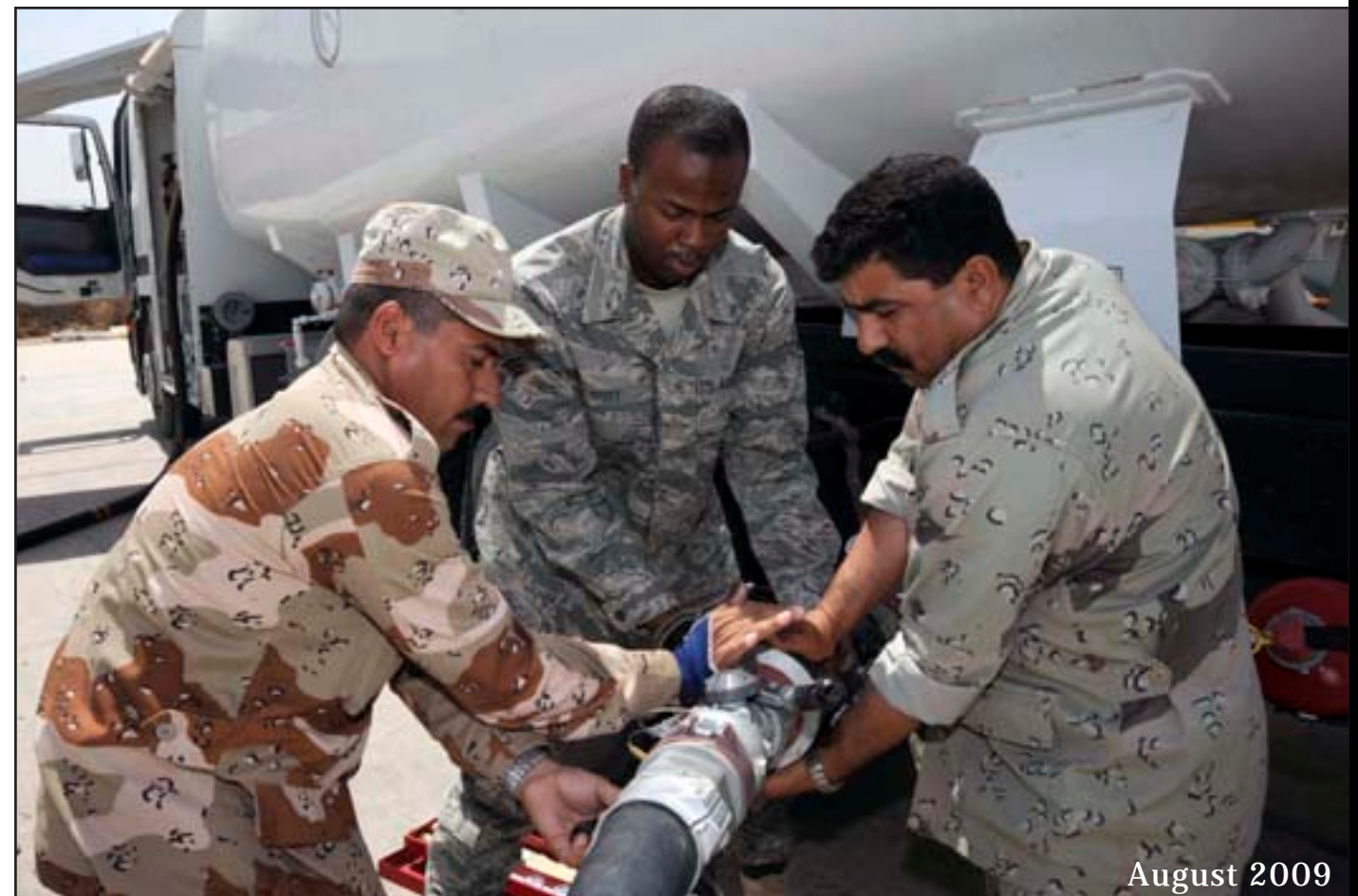
Below: Senior Airman David Britt, 447th Expeditionary Logistics Readiness Squadron fuels lab technician, and Iraqi air force members connect "Frankenstein" to an Iraqi fuel truck, July 20. "Frankenstein" is a fuel sampling connection built primarily by Britt, an Enterprise, Ala. native, to re-circulate fuel through the hose to the apparatus allowing an individual to safely retrieve a fuel sample. Britt is deployed from McConnell Air Force Base, Kan. (U.S. Air Force photo by Tech. Sgt. Johnny L. Saldivar)
