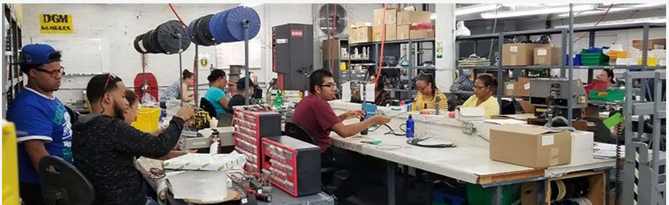
Roanwell employees prepare avionics cabling at the company's factory in the Bronx, New York.
