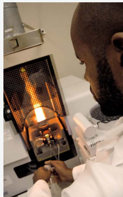
Andres Aquino, a Product Test Center-Analytical scientist, tests a metal sample in the atomic absorption spectrophotometer. PTC-A scientists use this equipment to analyze the concentration of elements in a liquid sample based on energy absorbed from certain wavelengths of light.
