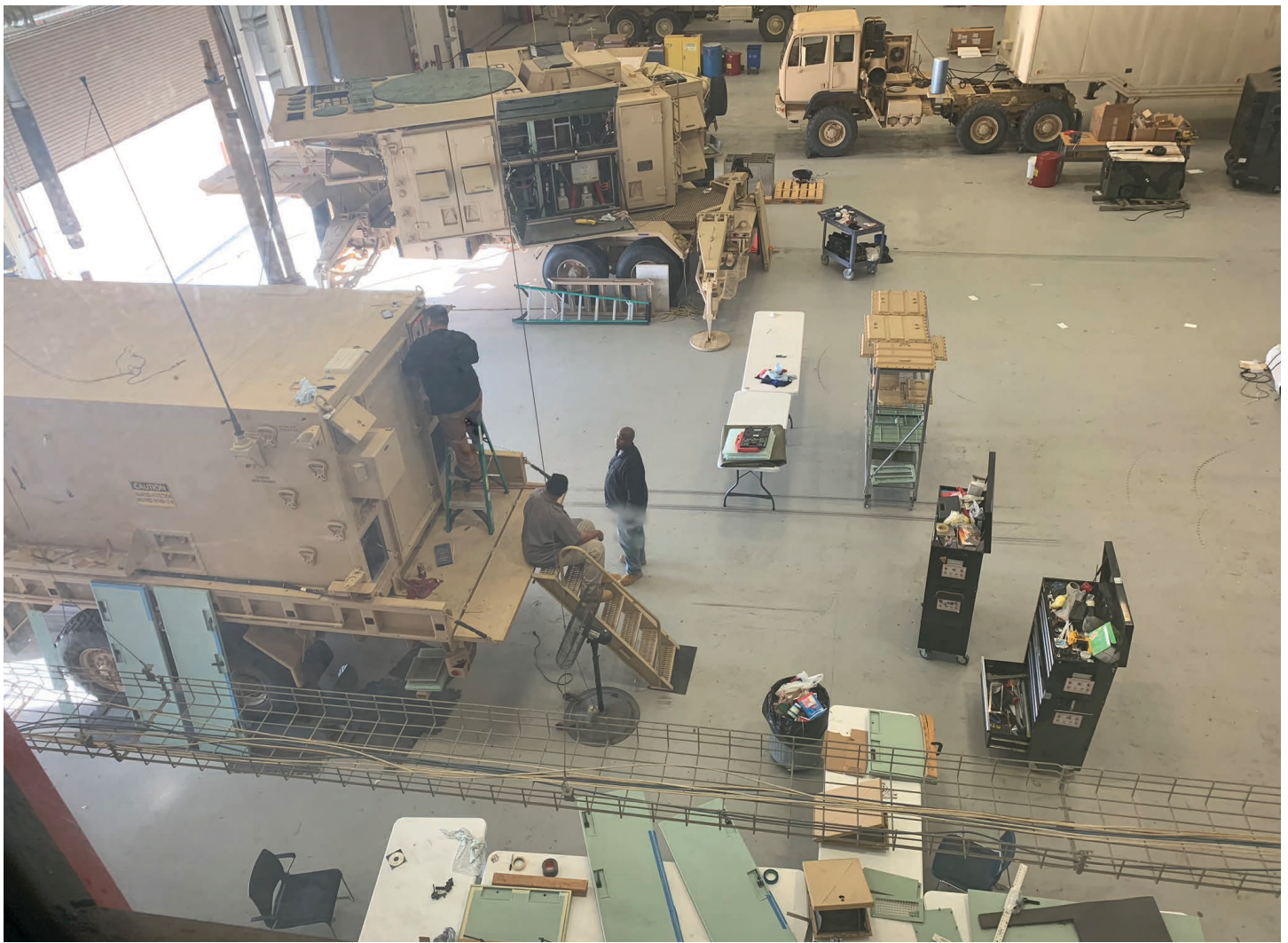
Raytheon contractors performed deep conventional maintenance and reset on an Engagement Control Station within the bay of the 3rd Battalion, 2nd Air Defense Artillery motor pool. (Chief Warrant Officer 3 Lewis Heck/U.S. Army)
