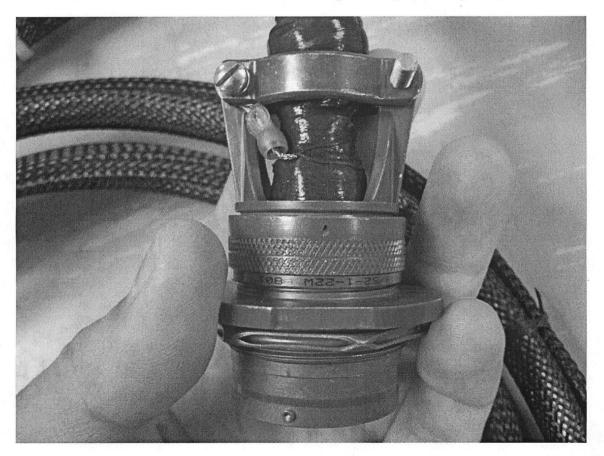
FIGURE #6 Properly Grounded terminal lug
