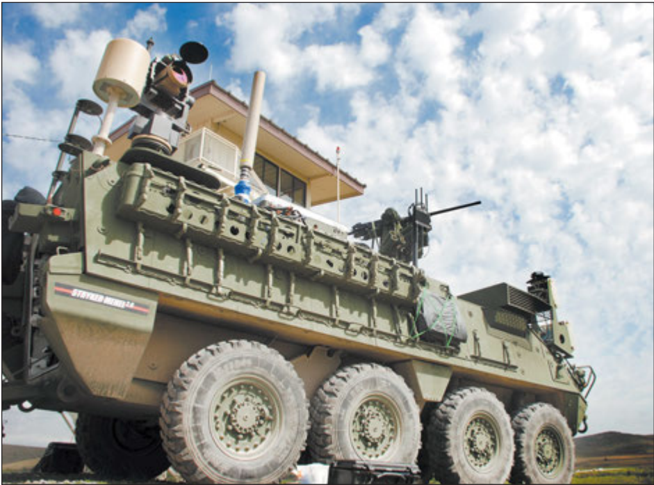
Monica Guthrie / U.S. Army During a test of the Maneuver Short-Range Air-Defense System, a 5-kilowatt laser is mounted on a Stryker armored vehicle during the Maneuver Fires Integrated Experiment known as MFIX at Fort Sill, Okla., April 5, 2017. The proposed FY20 budget funds the first MSHORAD battery, even though lasers will not be fielded on the vehicles until 2022.
