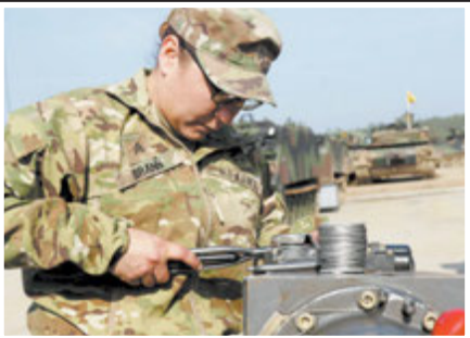
Sgt. Valarie Brann, a small arms and artillery repairer with 1-6 Infantry, repairs part of the cover of the M242 25mm gun chamber.
