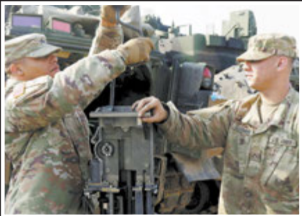
Sgt. Christopher Bell and Pfc. Damon Clemens clean an M242 25mm gun chamber for an M2 Bradley Fighting Vehicle.
