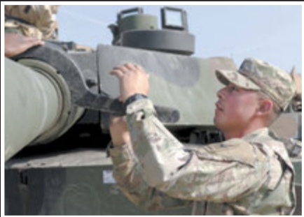
Staff Sgt. Brandon Telles uses a spanner wrench to tighten the gun chamber of an M1A2 Abrams tank after cleaning and lubricating it.
