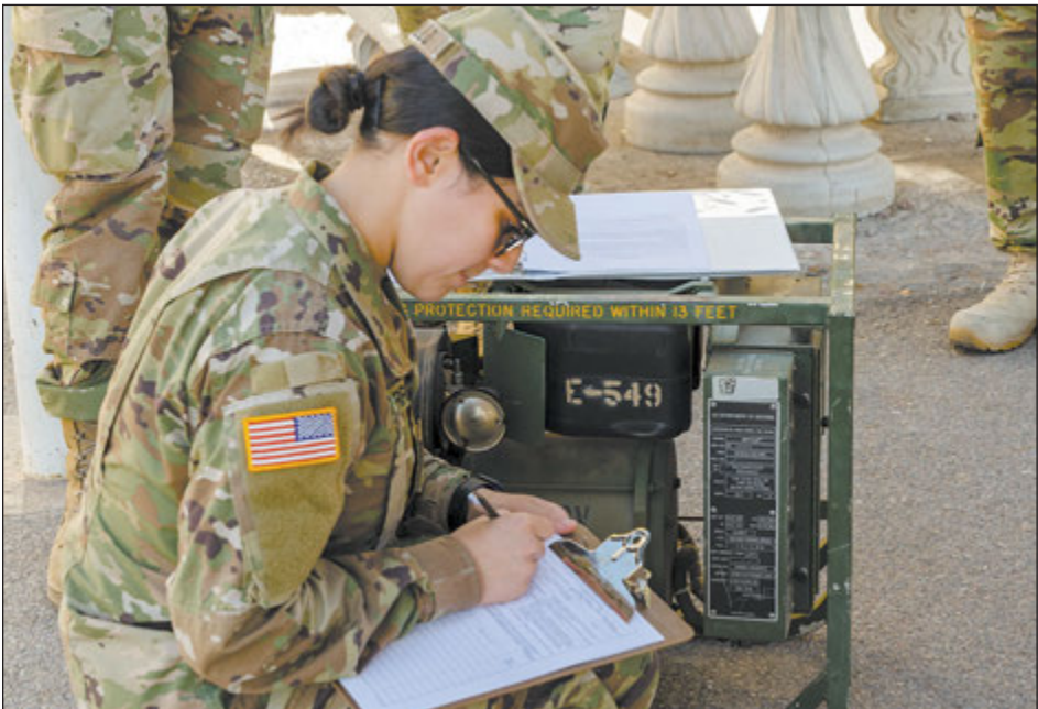
Capt. Joselyn Sydnor / Bliss MaD Bde./653rd RSG Sgt. Ivanska Carrillo, a 653rd Regional Support Group Soldier, notes deficiencies of a 2kW Military Tactical Generator Set as her group completes a block of instruction on Preventative Maintenance checks and services during training at Fort Bliss June 29.
