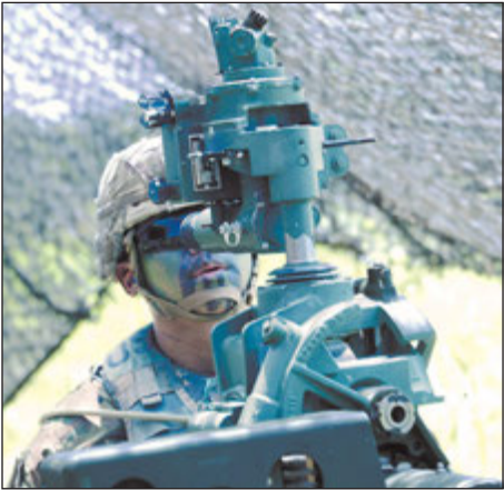
Sgt. Daniel Acosta uses the panoramic telescopic sight to position the M777 howitzer to fire for effect during degraded operations toward the end of a training exercise for Field Artillery AIT students on the west range of Fort Sill, Okla., June 19.
