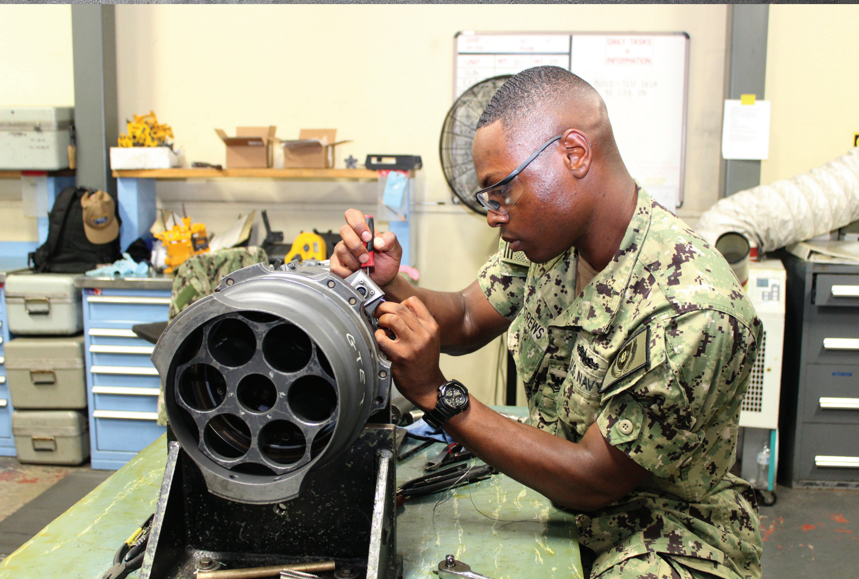
Fire Controlman 2 nd Class Terrance Andrews, Temporary Assigned to MARMC, finishes up his two week Gun Technician Enhancement Class by rebuilding a 20mm Closed In Weapon System Gun. (U.S. Navy Photo by Chris Wyatt/Released)
