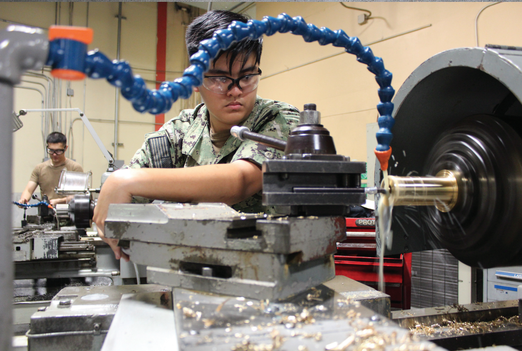
Machinery Repairman 3 rd Class Patrisha Castro using a lathe manufactures a hose adapter for the Diesel Shop. (U.S. Navy Photo by Chris Wyatt/Released)
