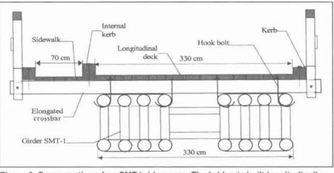
Figure 6. Cross section of an SMT bridge span. The bridge is built longitudinally with a wooden deck on crossbars.
