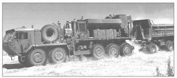
The versatility of the PLS system with EMMs is depicted in this photo of the EMM concrete mobile mixer with PLS dump body. Upon arrival at the work site, the PLS truck can off-load the concrete EMM for stationary operation, then load the dump body from the trailer to perform dump operations.
