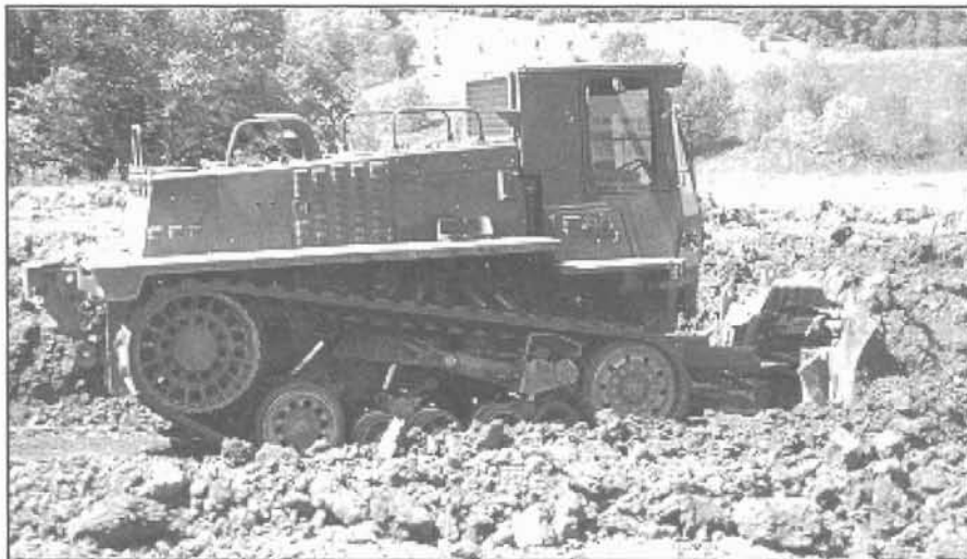
In the earthmoving mode, the DEUCE's blade can be tilted in six different positions with a joystick.
