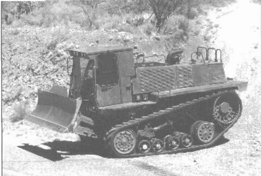
In the self-deploy mode, the DEUCE can travel up to 30 mph on asphalt roads without causing damage.
