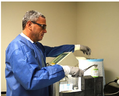
Jeff Kuehnhoff, radiopharmacist, puts a vial of lutetium Lu 177 dotatate into the dosage calibrator June 26, 2019, in the Nuclear Medicine Pharmacy. The dose calibrator calibrates the quantity of radiotracer activity in the radiopharmaceutical. This process is done to make sure the radiopharmaceutical is the accurate dose before it is administered to the patient. A dedicated radiopharmacist, who has had several years of additional training in nuclear medicine, handles these types of radiopharmaceuticals.
