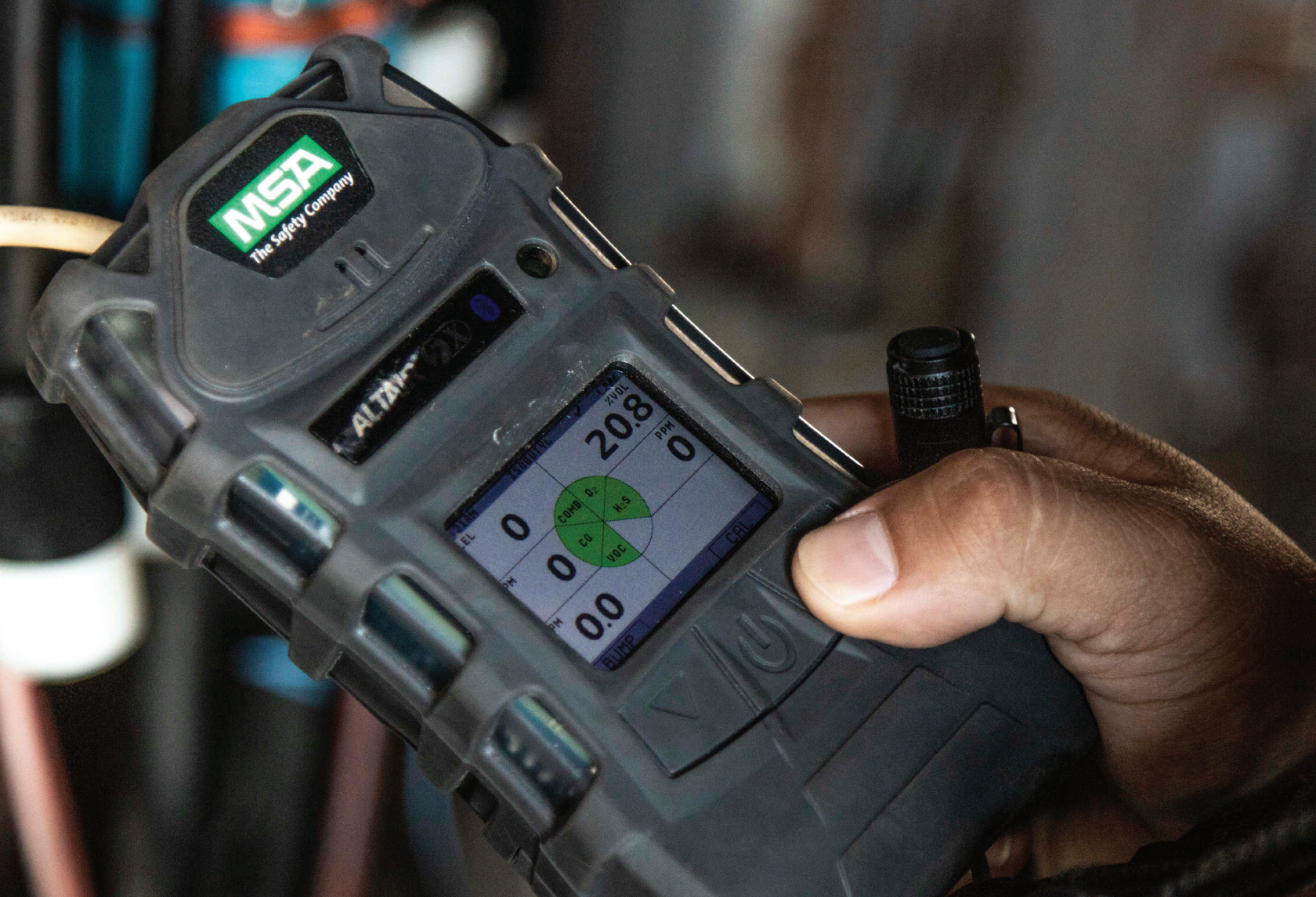
NORFOLK (July 9, 2019) Mid-Atlantic Regional Maintenance Center (MARMC) Navy Competent Person (NCP) Damage Controlman 2 nd Class Jesus Figueroa tests a confined space prior to entry aboard USS Laboon (DDG 58), which is currently pier side at Naval Station Norfolk. (US Navy Photo by Derry Todd/Released)
