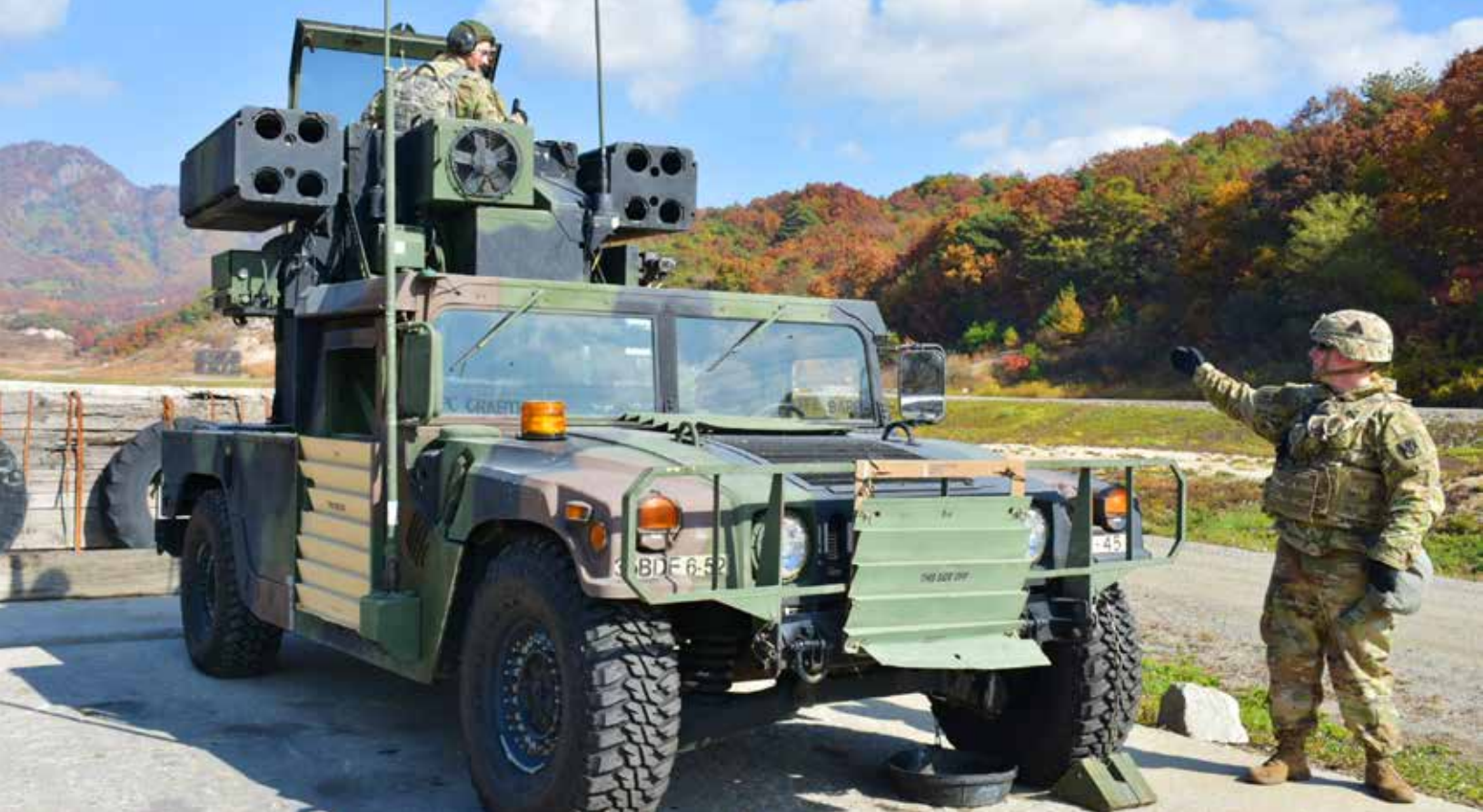
Team Chief Sgt. Justin Adams verifies bore sight adjustments on the M3P .50 caliber machine gun with the assistance of the 94T Avenger System Repairer, Pfc. Jason Talbot. » U.S. ARMY PHOTO BY: 2ND LT. BRAY MCCOLLUM, ECHO BATTERY, 6-52 AIR AND MISSILE DEFENSE BATTALION
