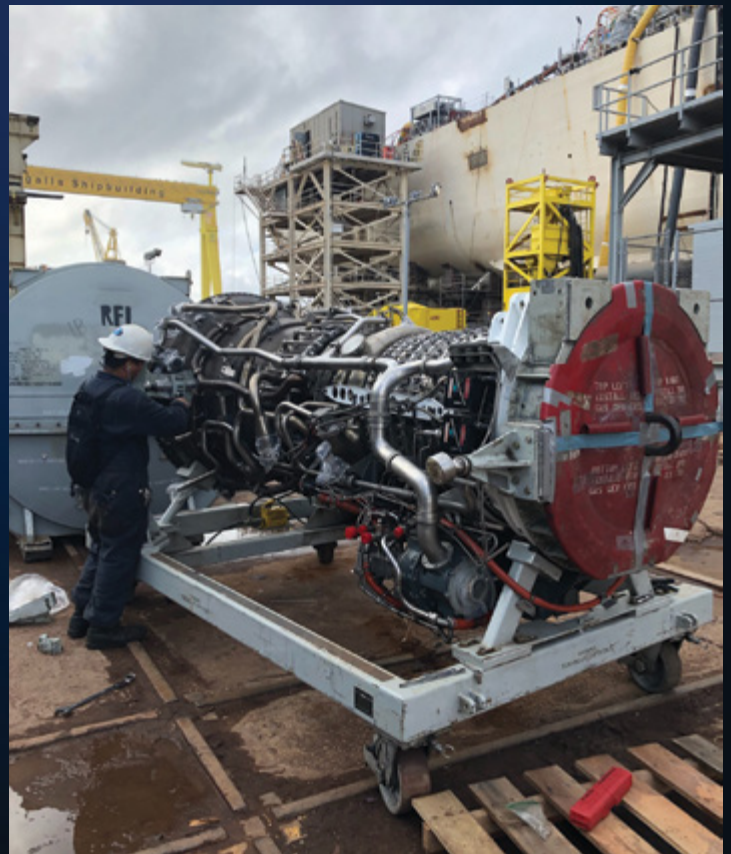
NORFOLK (Feb. 15, 2019) A MARMC Sailor finishes attaching loft fixtures on an LM2500 Gas Turbine Main Engine prior to it being hoisted by a crane for installation. (U.S. Navy photo by MARMC personnel/Released)
