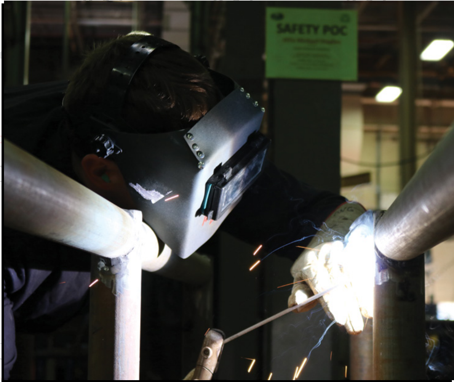
Hull Maintenance Technician 2 nd Class Chase Hicks stick-welds a galvanized steel rack for metal storage in the Hull Shop (U.S. Navy photo by Damage Controlman 3 rd Class Hannah Sweet/released)
