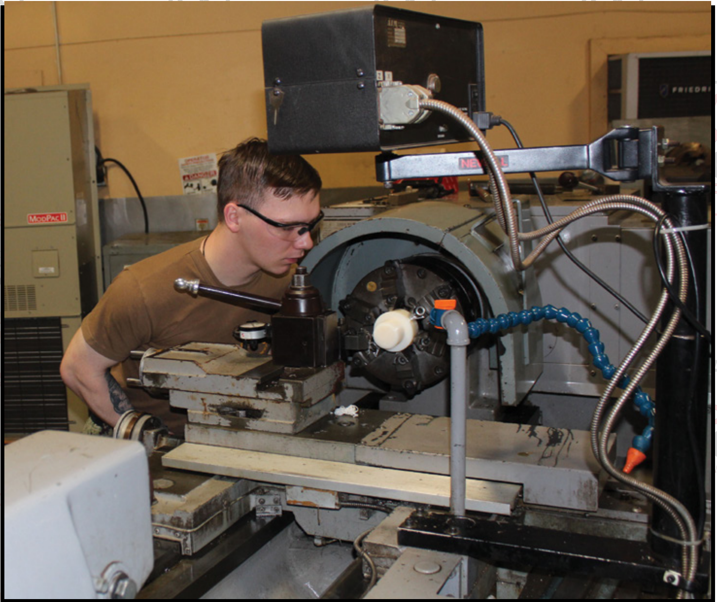
Mid-Atlantic Regional Maintenance Center Inside Machine Shop's Machinery Repairman Fireman Christopher Hood threads nylon plugs which are used on USS Carter Hall (LSD 50) flight deck. (U.S. Navy photo by Chris Wyatt/Released)
