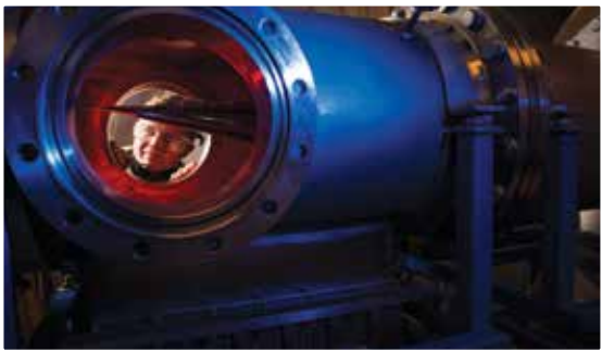
(U.S. Air Force photo by Joshua Armstrong) Cadet 2nd Class Eric Hembling uses a Ludwig Tube to measure the pressure, temperature and flow field of various basic geometric and hypersonic research vehicles at Mach 6 in the U.S. Air Force Academy's Department of Aeronautics, Jan. 31, 2019.
