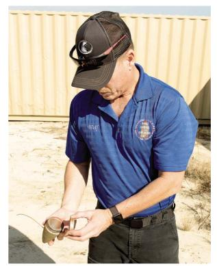
Wolf Amacker, Fort Bragg installation range officer, inspects the nose cone of a 2.75 inch rocket that was fired on the new aerial gunnery range. The rocket contained approximately 2,200 20 grain flechettes. Flechettes are small steel darts that disperse in front of a target and then penetrate vehicles and light armor.
