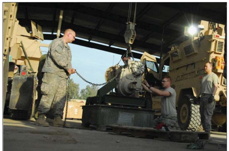
Mechanics from B Co. -- Bonecrusher -- 1-161 st Inf. (CAB) lower a Medium Tactical Vehicle transmission into a crate at Joint Base Balad, Iraq before shipping to depot to be rebuilt. (Photo by Sgt. David Isaac)
