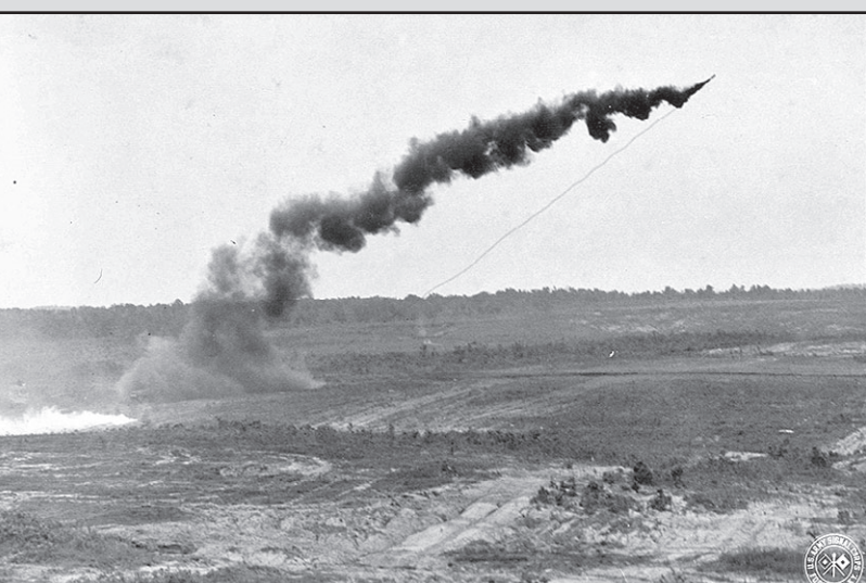
Reaching where tanks couldn't, a rocket propelled line-charge was electrically fired to a predetermined point where the detonated blast could clear a 10 foot wide path through mine fields or vegetation. The results of this test rattled homes up to 30 miles away.
