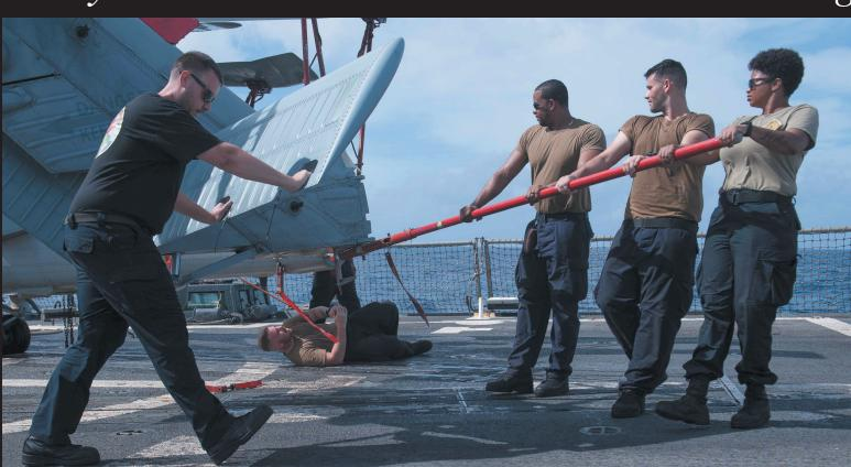
Sailors fold the tail cone section of an MH-60R Sea Hawk, with Helicopter Maritime Strike Squadron 37, aboard the Arleigh Burke-class guidedmissile destroyer USS Chung-Hoon (DDG 93), Nov. 20.
