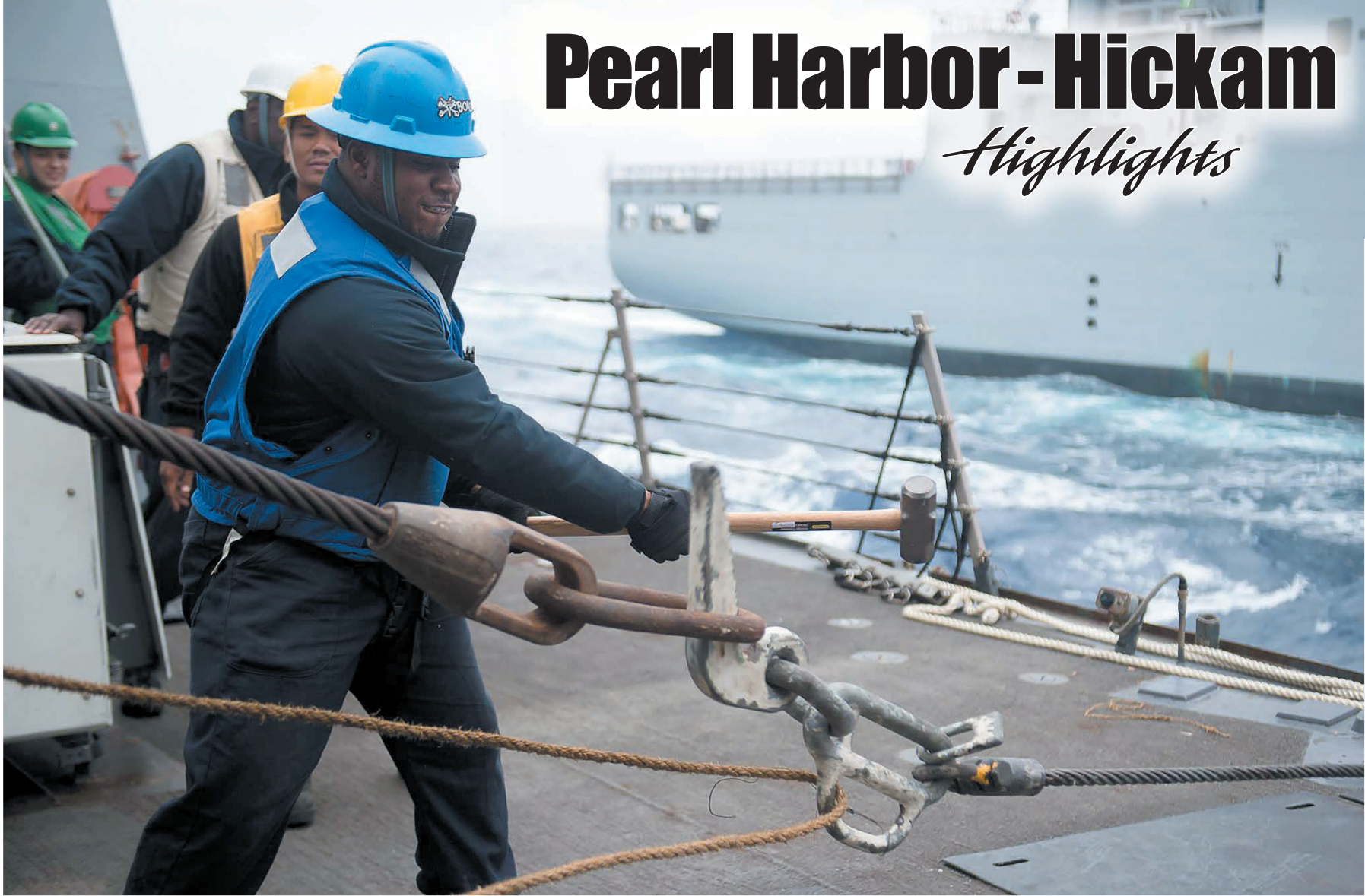
U.S. Navy photo by MC3 Logan C. Kellums Seaman Davion Gayle, from Jamaica, assigned to the Arleigh Burke-class guided-missile destroyer USS Chung-Hoon (DDG 93), uses a hammer to disassemble a pelican hook during a replenishment-at-sea with the Lewis and Clark-class dry cargo and ammunition ship USNS Charles Drew (T-AKE 10), Aug. 20.
