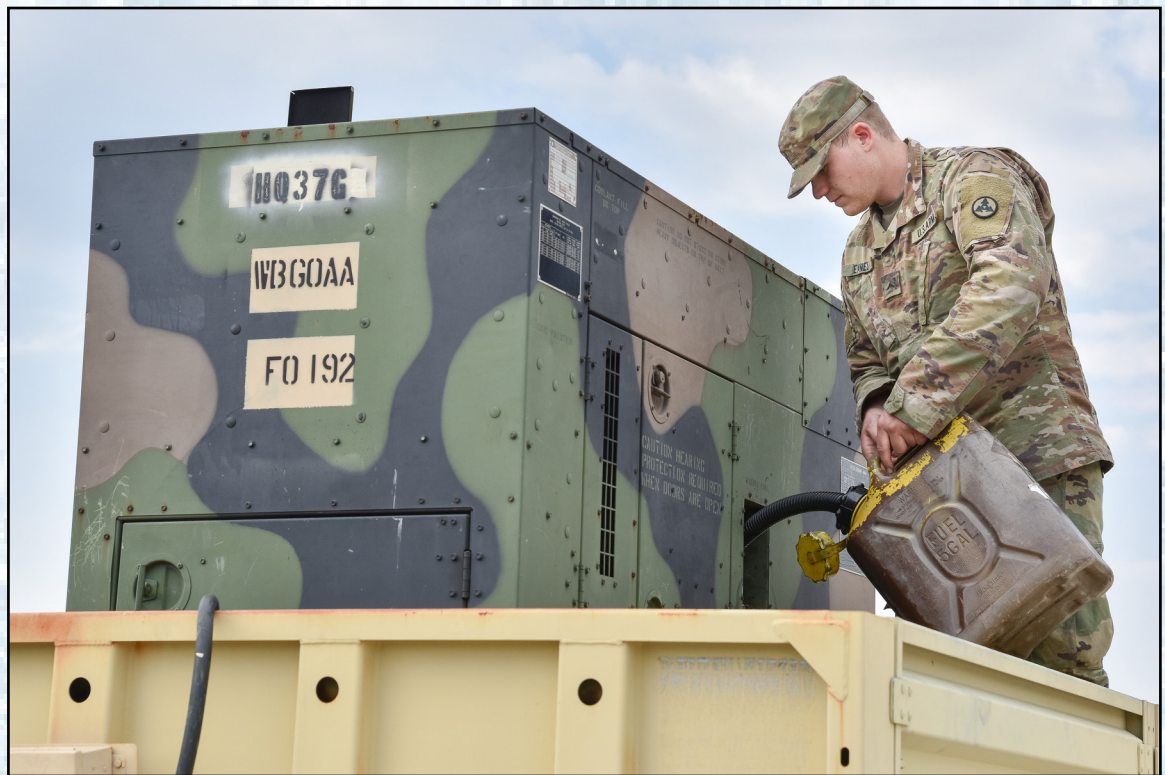
The Containerized Ice Making System, or CIMS, was developed by the Product Manager -- Force Sustainment Systems, and can successfully generate and bag 3,600 pounds of potable ice per day and keep 1,200 pounds in cold storage for future use. The CIMS' capacity to produce on-demand ice meets the field feeding, medical, and mortuary affairs needs of Soldiers fighting down range. Two third generation prototype CIMS units were brought in to support the XVIII Airborne Corps' 3rd Expeditionary Support Command during a training exercise held at Fort Bragg in April 2018. (Photo Credit: Jeff Sisto, NSRDEC).
