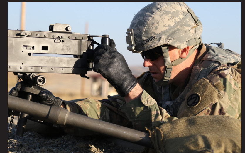
Staff Sgt. Jeff Harley, petroleum supply specialist, 842nd Quartermaster Company, adjusts a traversing and elevation mechanism on an M2 machine gun during Operation Cold Steel II, Oct. 15, 2017.
