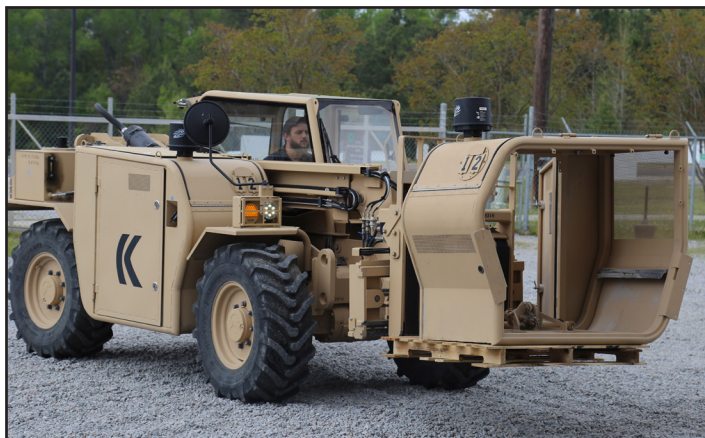
The M5K Forklift is another technologically improved piece of equipment that improves the capability of Army units as well as AMSA and ECS because of increased dexterity.
