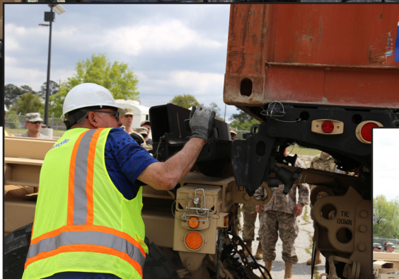
Members of Kellogg, Brown and Root help Charlie Johnson demonstrate a new bracket that allows the Palletized Loading System to transport CONEX containers without loading them on a flat rack. (Photos by Sgt. 1st Class Jeff Mullett)
