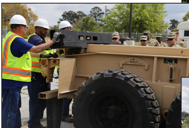
Members of Kellogg, Brown and Root help Charlie Johnson demonstrate a new bracket that allows the Palletized Loading System to transport CONEX containers without loading them on a flat rack. (Photos by Sgt. 1st Class Jeff Mullett)
