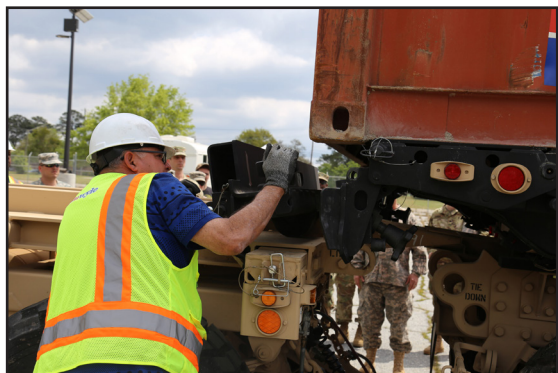
KBR personnel demonstrate how the new bracket mounts to the rear of a Conex Container making it work on the PLS trailer without a flat rack.
