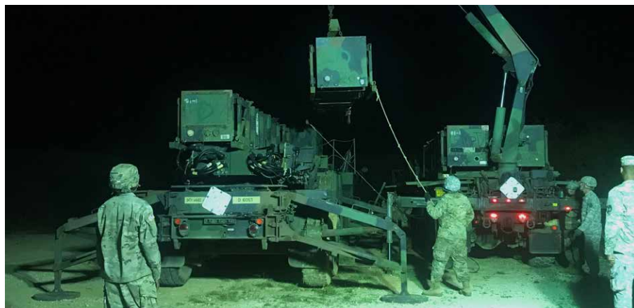
Soldiers with Delta Battery, 1st Battalion, 1st Air Defense Artillery Regiment performs launcher reloading drills using the M985A4 Guided Missile Transporter (GMT). » PHOTOS COURTESY: U.S. ARMY
