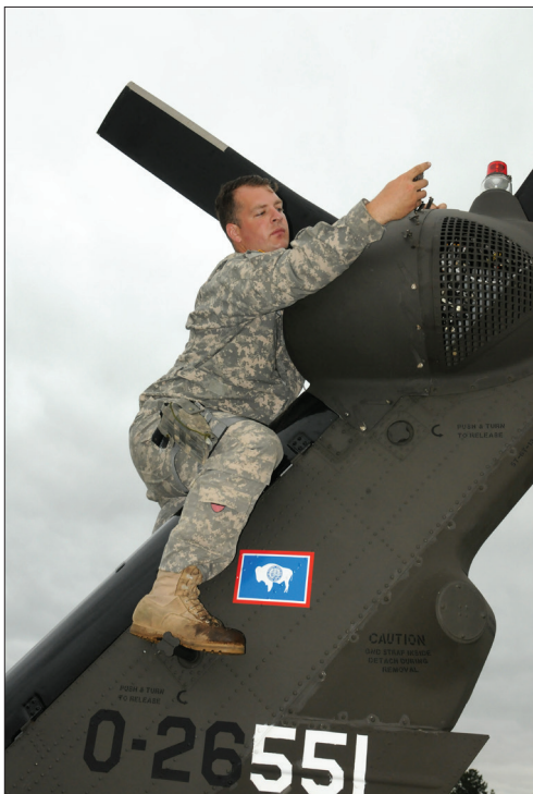
U.S. Army Sgt. Jordan Wisdorf, a crew chief with G Company, 2nd Battalion, 211th Aviation Regiment, unscrews the fittings for a cover on a UH-60 Blackhawk helicopter, part of a pre-flight inspection during the Golden Coyote exercise, Custer State Park, South Dakota, June. (U.S. Army photo by Sgt. Jack Eden)
