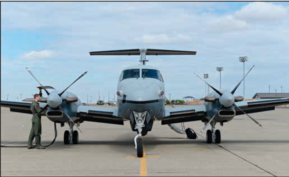
U.S. Air Force photo by Airman 1st Class Ramon A. Adelan Capt. Sam, 427th Reconnaissance Squadron MC-12W Liberty pilot, inspects the aircraft before takeoff Sept. 16, 2015, at Beale Air Force Base, California. Sam and other Beale Airmen conducted the aircraft's final flight with Air Combat Command. The MC-12W is a medium- to low-altitude, twin-engine turboprop aircraft, which provides intelligence, surveillance and reconnaissance support directly to ground forces.
