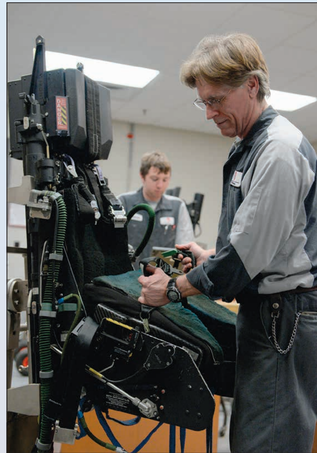
Roy Norman, L3 Technologies T-38C Talon egress mechanic installs a survival kit onto a T-38 ejection seat, Feb. 14, 2018, on Columbus Air Force Base, Mississippi. After the final inspection of each T-38 seat the survival kit is reinstalled, this process ensures the seat is up to date and ready to be used in case of an emergency.
