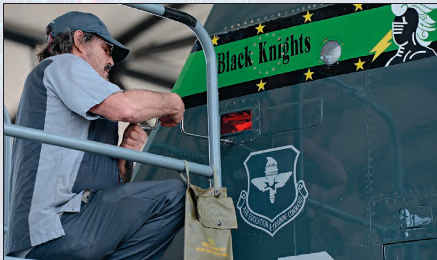
Raymond Beauregard, L3 Technologies senior aircraft maintainer, tightens screws after repairing the rotating beacon on a T-38C Talon Feb. 15, 2018, on Columbus Air Force Base, Mississippi. Routine maintenance can be completed on the flight line, and is essential for quickly getting aircraft back into the air. Larger fixes are towed to one of the many hangers on Columbus AFB and are repaired day and night until completed.
