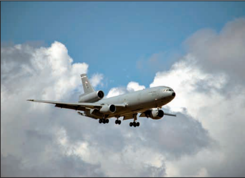
U.S. Air Force photo by Tech. Sgt. Heather Redman A KC-10 Extender, from Travis Air Force Base, California, prepares for landing at Joint Base Pearl Harbor-Hickam, Hawaii, Oct. 30, 2017. Using either an advanced aerial refueling boom, or a hose and drogue centerline refueling system, the KC-10 can refuel a wide variety of U.S. and allied military aircraft within the same mission.
