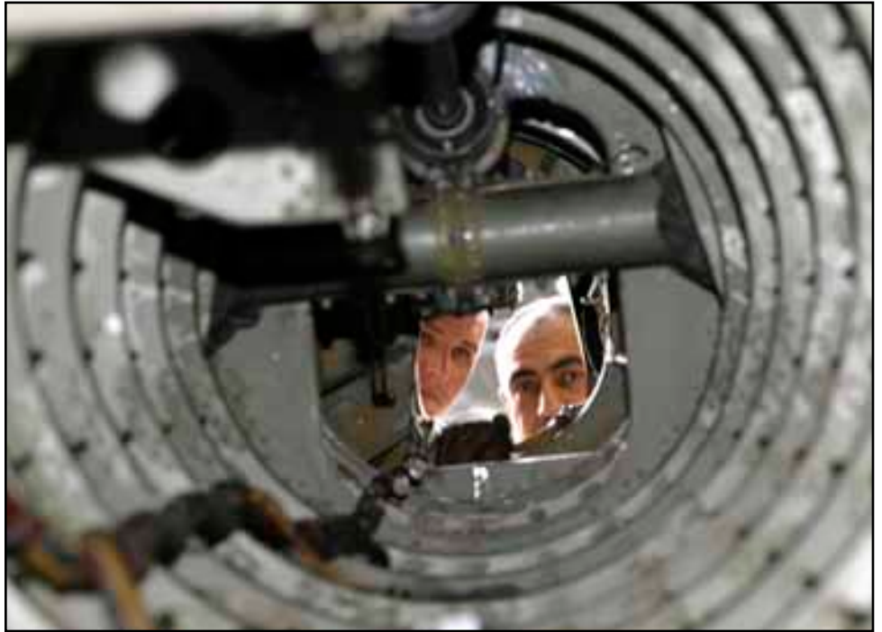
ALL PHOTOS: U.S. Air Force Tech. Sgt. Lee Everhart and Iraqi Air Force Lt. Col. Auday Yassen Youssif perform maintenance on a Mi-17 Hip helicopter in a hangar at Taji Air Base, Iraq, Sept. 11. The helicopter made a hard landing and struck its tail skid against the ground during a training mission, requiring a close inspection of its tail section.
