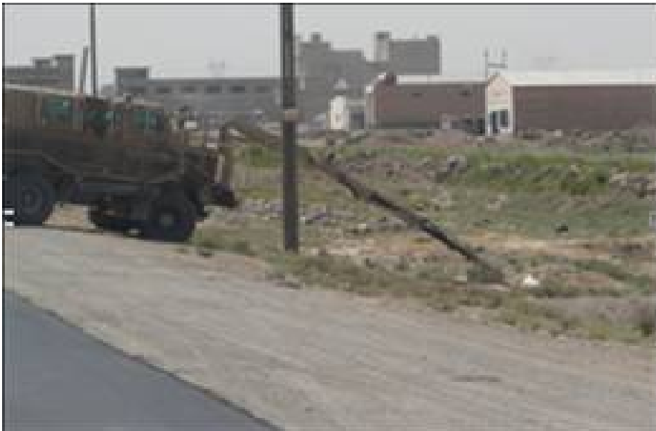
Bravo Company, 40 th Engineer Battalion, Task Force Ram's Buffalo interrogates a suspicious item utilizing the Buffalo's spork during one of their many route clearance missions.(U.S. Army Courtesy photo)
