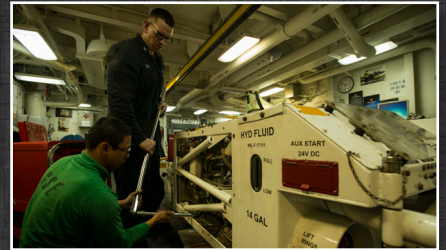
AS2 John Ruiz and AS2 Darwin Payawal install a hydraulic pump in an A/S32A-32 spotting dolly in the hangar bay during a routine patrol off the waters south of Japan. (Photo by MC2 Janweb Lagazo)
