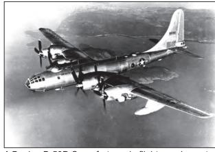
A Boeing B-50D Superfortress in flight wearing natural metal. The larger tail of the B-50 compared to the original B-29 can be seen here.
