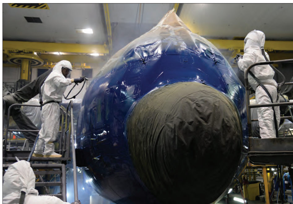
576th Aircraft Maintenance Squadron painters apply a second coat of blue paint on the fuselage of Fat Albert on May 17 at Hill Air Force Base, Utah. The aircraft received a new paint job following a major eight-month, depot-level maintenance overhaul.
