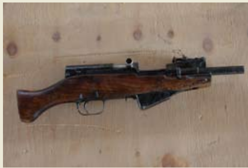
A pistol made from a cut down, Russian-designed SKS 7.62x39 mm rifle.
