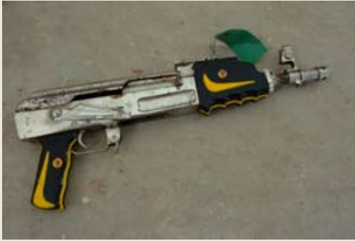
A pistol made from an AK-47 rifle. The buttstock has been removed, the barrel shortened and the pistol grip and handguard have been replaced.
