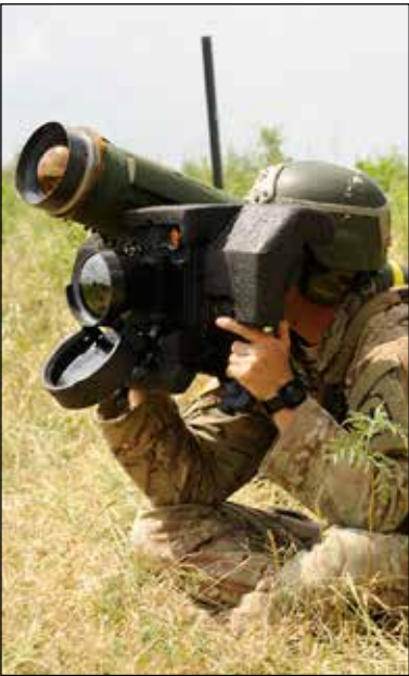
Target Set-Up: A Nebraska Soldiers takes aim with an FGM-148 Javelin. The FGM-148 Javelin is a “fire-and-forget” missile. Soldiers lock onto their target before launch and rely on the automatic self-guidance system to reach its intended destination.
