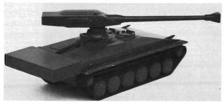
Fig 1b. (Above) Model of the Swedish UDES-40 shows crew-in-hull layout with yoke-mounted external 120-mm gun, fed by external magazines at the rear of the hull.
