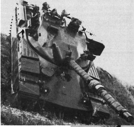
Styles in thermal sleeves vary, with British, above, wrapping their gun tubes in a sort of tarpaulin jacket, while U.S. tanks like the M60, right, and Soviet T-72, below, use rigid insulating sleeves held on by metal bands. A snug fit is essential for accuracy, the author says.
