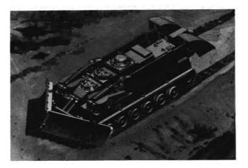
The counterobstacle vehicle, showing its 'dozer blade, excavating buckets on the rear and other changes to the basic *M88A1* chassis. The vehicle will undergo a six-month test period beginning in July.
