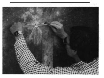
An Aberdeen technician measures penetration and diameter of a hit on armor plate made by an AT4 rocket from the new antiarmor weapon now under test at the Proving Ground in Maryland. The AT4 is said to penetrate 450-mm of armor.
