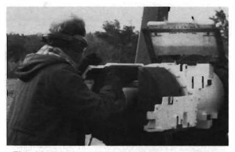
The ultimate test — a special over-pressure 105-mm round is pushed into the breech of a gun under test. The round will exert internal pressures up to 113 percent over the gun's designed safety factor. After testing, the gun and ancillary mechanisms are stripped down, examined and reassembled to complete the test sequence.
