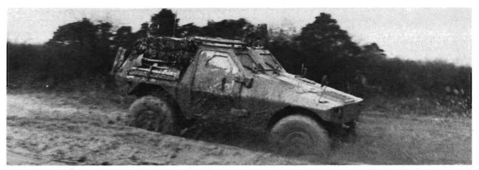
The M11's low ground pressure of 11 lbs. per square inch enables it to move over soft ground with ease. Reduction gears at each wheel have the effect of increasing ground clearance without adding additional height to the vehicle.
