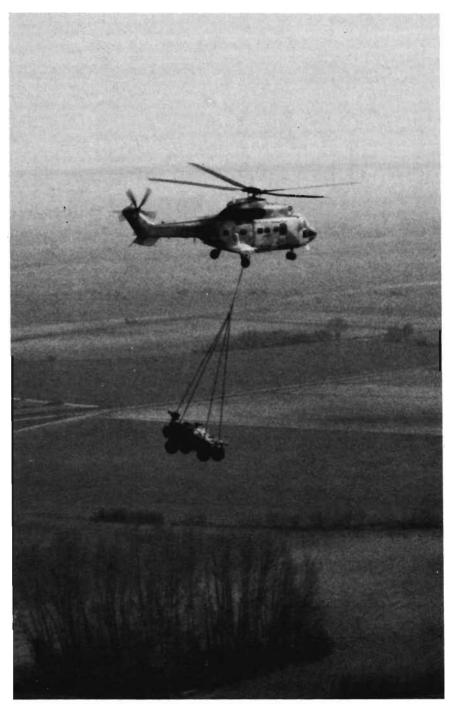
The M11's low weight, 6,285 pounds unloaded and 7,807 pounds combat loaded, can be easily lifted by a variety of helicopters and fixed-wing aircraft. Panhard foresees development of a broad family of 24 versions of this basic vehicle.
