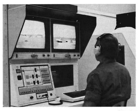
A technician at the evaluator's station sees both commander's and gunner's views on TV monitors. View on right hand screen is a magnified section of same view on screen at left.
