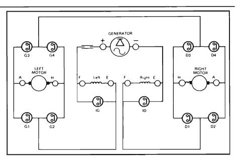
Electrical schematic of the ACEC drive system for armored vehicles.
