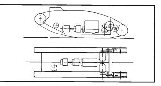
Electric current from a generator, rather than mechanical torque, moves through a cable to electric motors located at each drive sprocket, at a considerable saving in weight and volume. This permits improvements in the general appearance and compactness of the vehicle. Reversing the present circle in armor design permits the following advantages:
