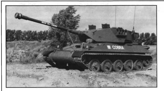
The Cobra 90 light tank, above, and the Cobra 41 APC, at right, are both powered by electric drives, but the powered sprockets are at the rear on the APC and at the front on the The Cobra 90. two vehicles illustrate the flexibility of layout poswith electrical sible drive. A diesel engine drives the electrical generators in both vehicles.
