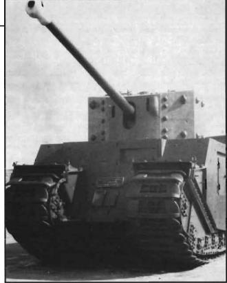
The TOG, a WWII-era British tank design, used an electrical power transmission system, but was never produced for combat use.
