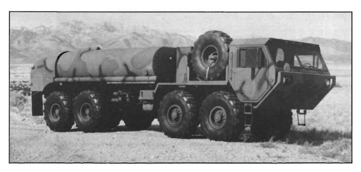
HEMTT fueler's design permits refueling two vehicles at once, on either side.
