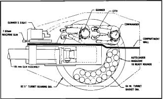
A major change in the AGS is the elimination of one crew member in favor of an automatic loader, seen at left. In sketch above, note compartment wall that separates and protects two turret crewmembers from autoloader mechanism.
