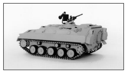
Above, two views of a model illustrating author's concept for an airborne IFV based on a shortened Bradley chassis. Javelin missile and ASP 30-mm cannon provide firepower.
