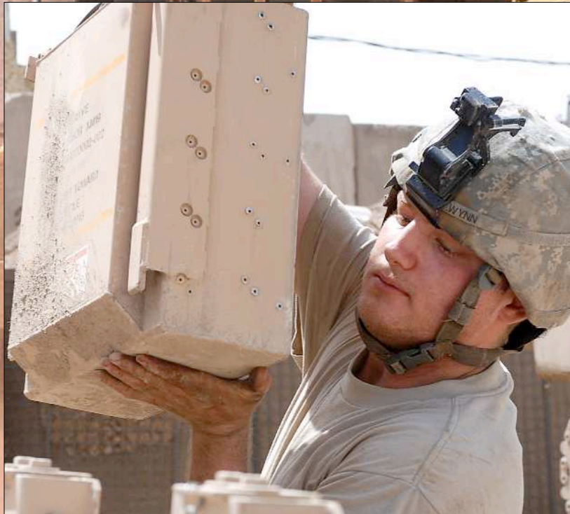
Photos by Spc. Joseph Rivera Rebolledo Pfc. Brandon Wynn puts a tank reactive tile in place in order to close the tank's skirt and finish track maintenance on his M1-A2 Abrams tank at Combat Outpost Ford in northeast Baghdad. Wynn serves as a tanker with Company C, 1st Combined Arms Battalion, 68th Armor Regiment, 3rd Brigade Combat Team, 4th Infantry Division.
