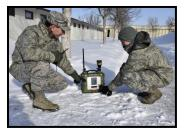
Senior Master Sgt. Amber Westie waves gasoline beneath the sensor of the Area RAE pro, a long range contaminant detection monitor while Tech. Sgt. Marcus Jackson, 120th Airlift Wing readiness and emergency management flight specialist, verifies the alarm was tripped. (U.S. Air National Guard photo/Staff Sgt. Lindsey Soulsby)
