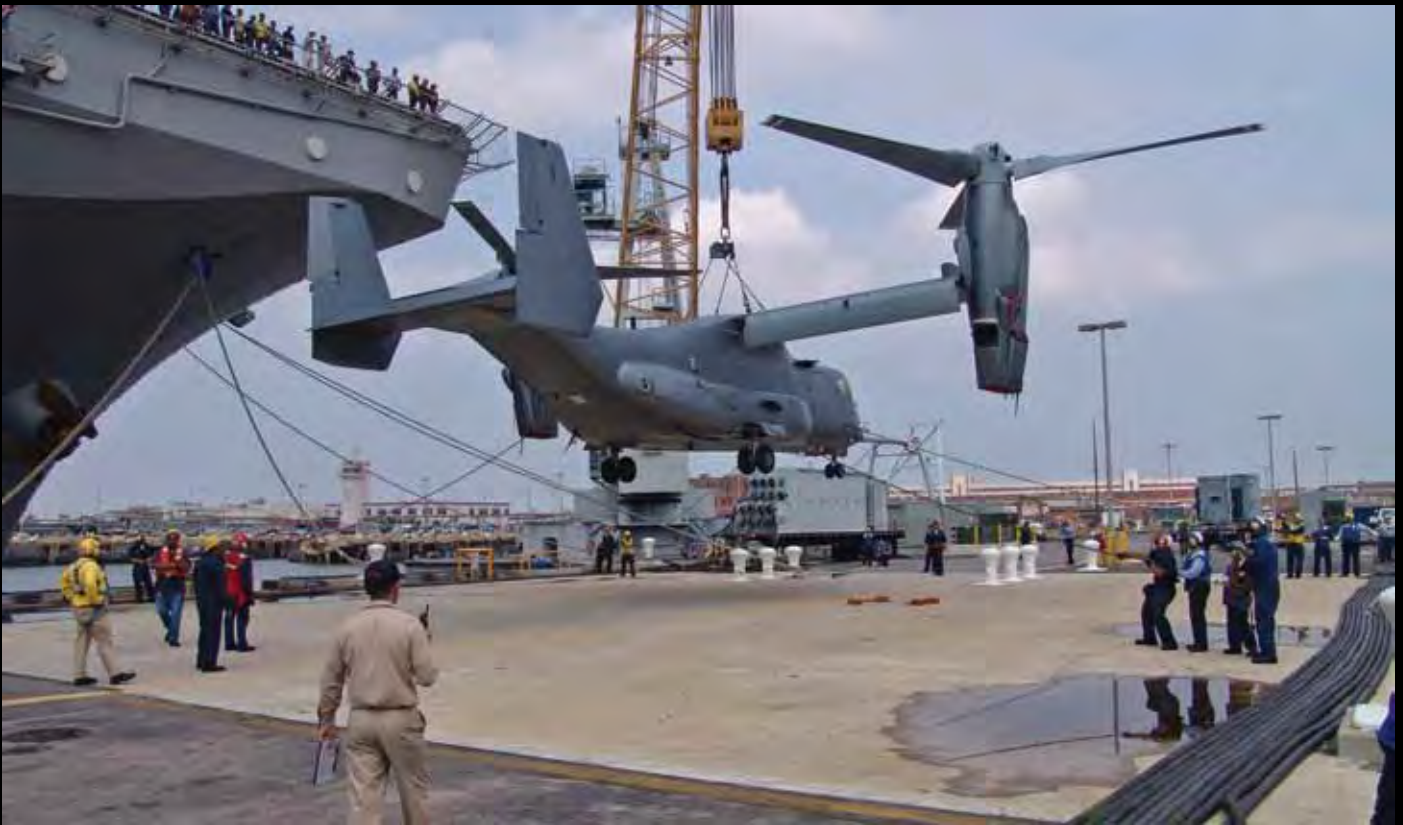
An MV-22 Osprey being hoisted by a crane onto a flight deck.
