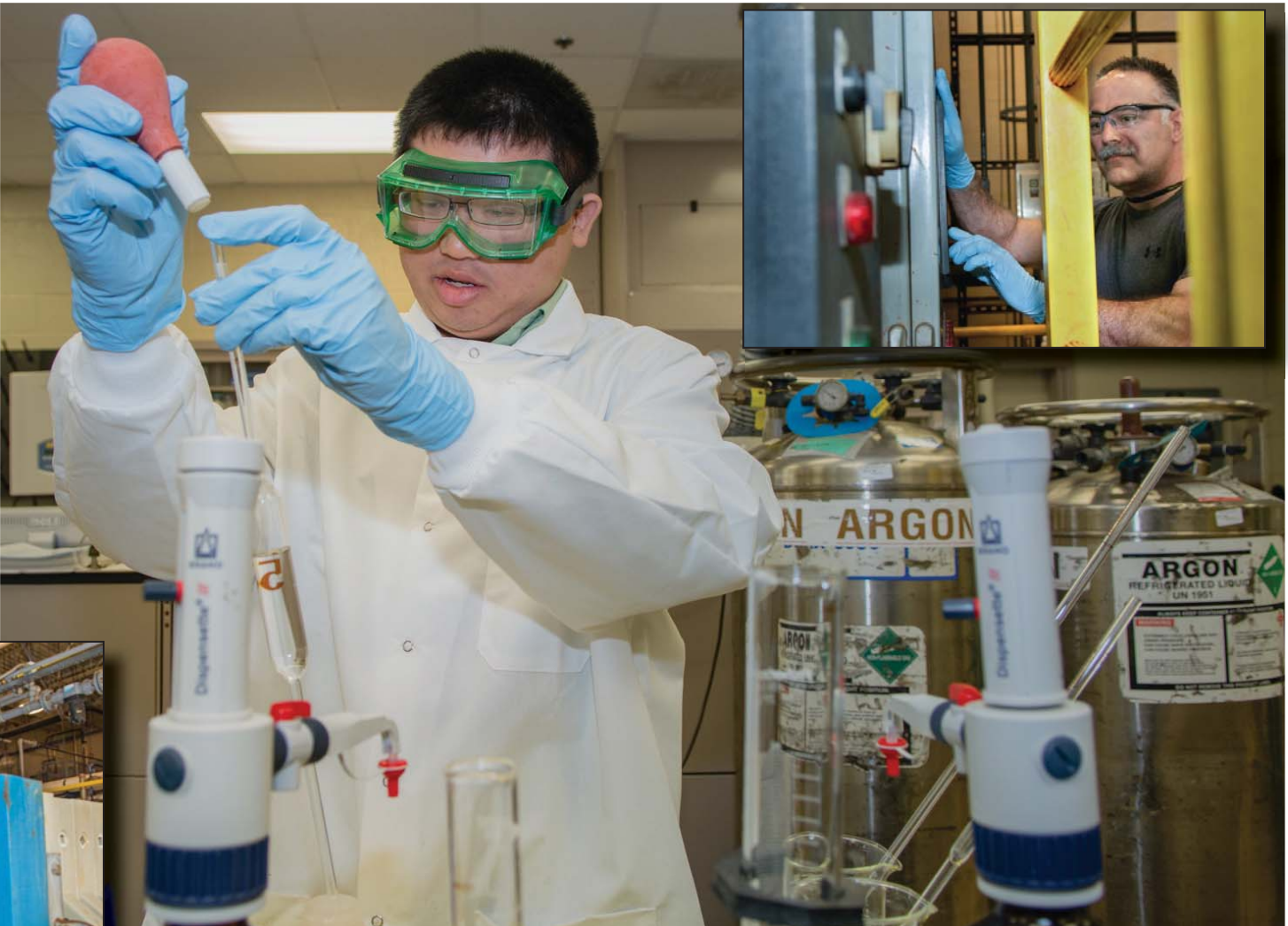
Bobby Diep, chemical engineer, performs chemical analysis on electroplating process solutions. INSET, Chas Valenza, chemist and lead engineer, programs process adjustments into the reverse osmosis (RO) system. RO is used to purify and recycle contaminated wastewater from electroplating operations to minimize cost and conserve natural resources.
