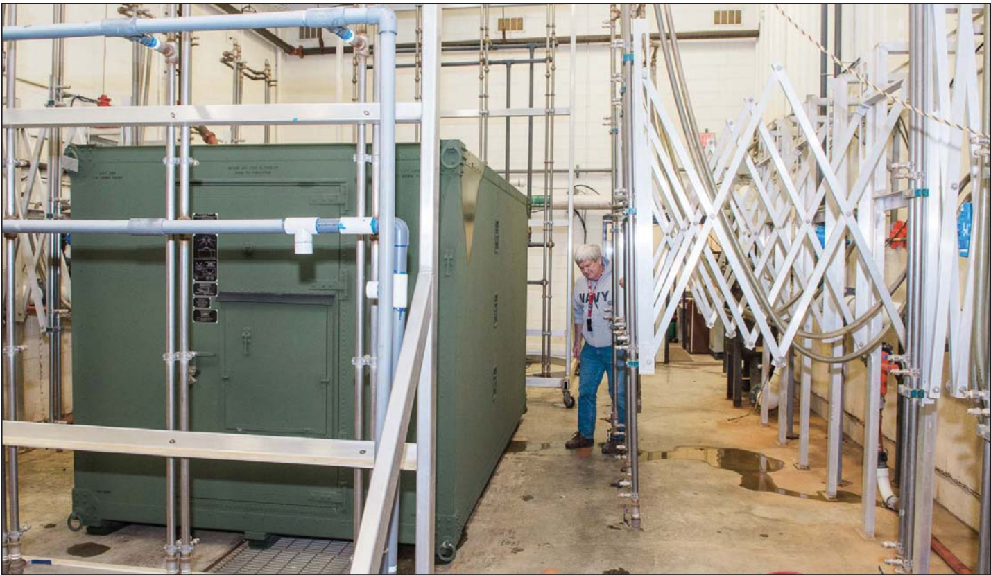
Clockwise: Edward Pitcavage, finish inspector, makes sure nozzles are the correct distance from a shelter before it starts to rain in the depot's rain test facility (top right), which is used to check the water tightness of equipment repaired or overhauled here. Right, Pitcavage confirms specific nozzles are selected according to customer requirements. Pitcavage works in the Continuous Process Improvement Directorate's Quality Control Division.
