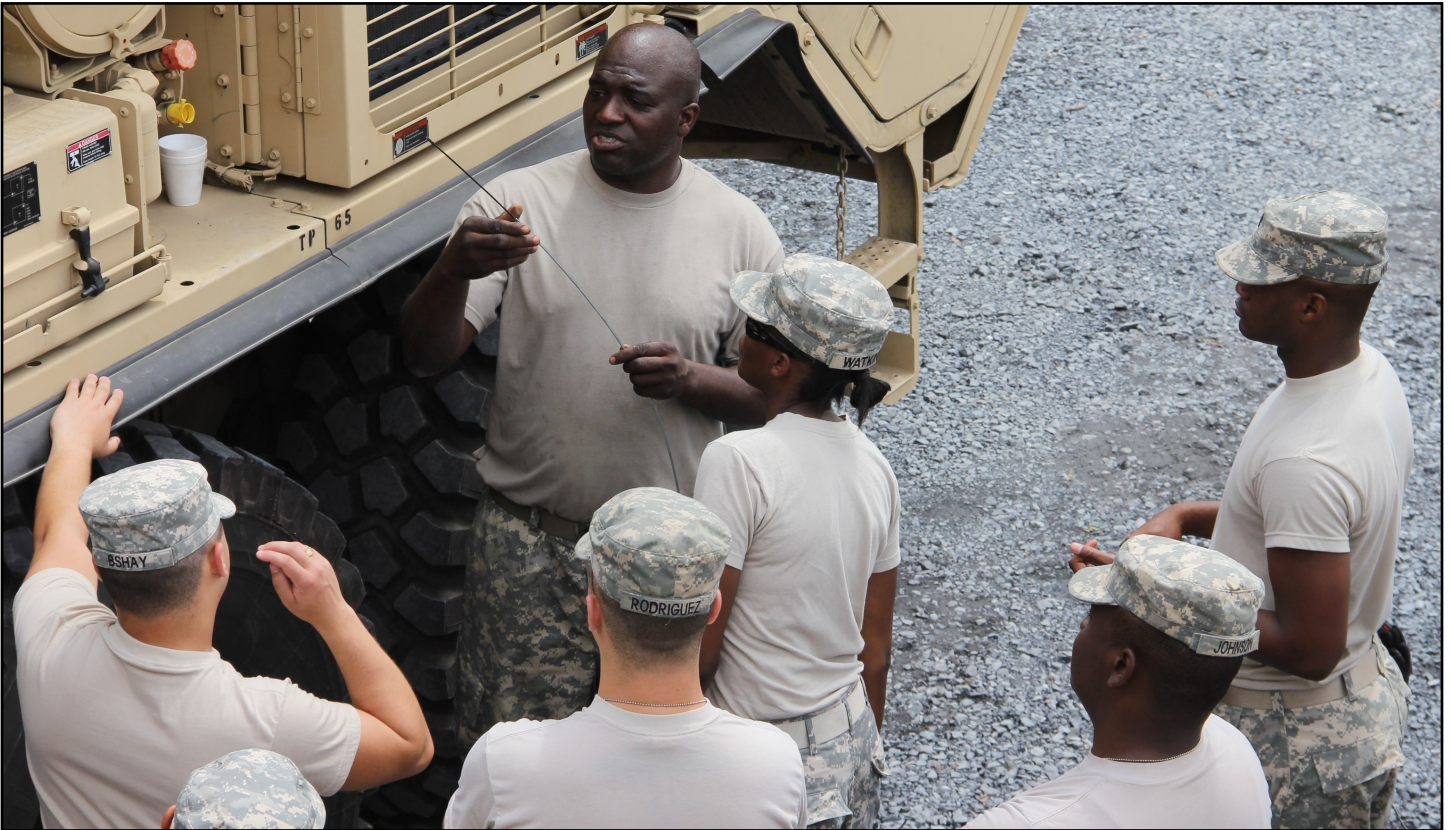
Staff Sgt. James Weathers, top center, motor transport operator, shows Soldiers of the 1067th Transportation Co. how to check fluid levels as part of preventative maintenance checks and services on the M1075 Palletized Load System on Aug. 2, 2016 at Fort Indiantown Gap, Pa. (U.S. Army National Guard photo by Sgt. Jason Fetterolf)
