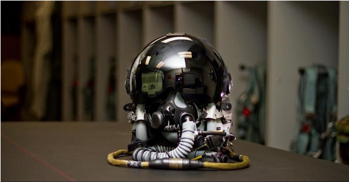
The Helmet Mounted Integrated Targeting [HMIT] system has given ANG F-16s a force-multiplying cueing system that allows the pilot to acquire targets just by looking at them. (USAF/NJANG)
