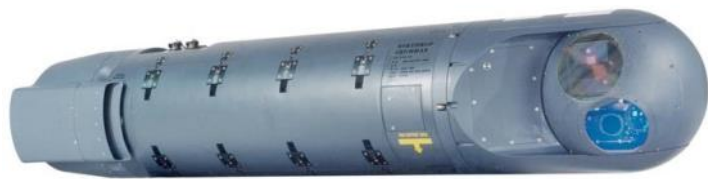
The compact LITENING advanced targeting pod has replaced the earlier LANTIRN two-pod system. (Northrop Grumman)
