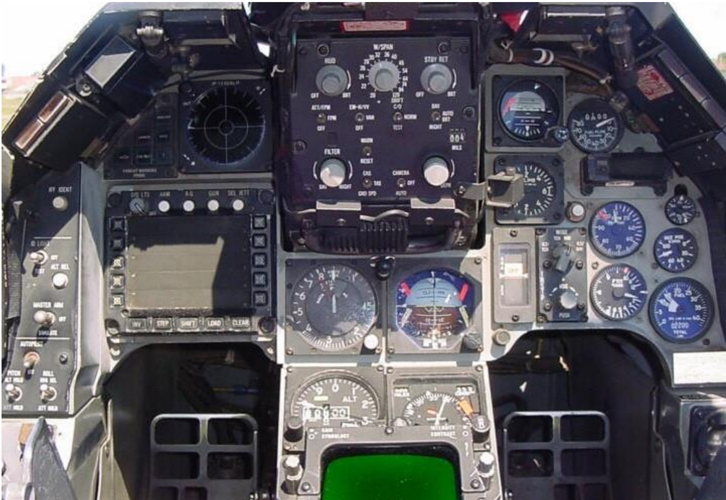
The instrument panel of the original YF-16 was typical of its day – “steam gauges” dominate the pilot’s view. (General Dynamics via F16.net)
