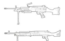
**M-249 Squad Automatic Weapon** – A lightweight, gasoperated, one-man-portable automatic weapon capable of delivering a large volume of effective fire at ranges up to 800 meters. Two M249s are issued per infantry squad.
