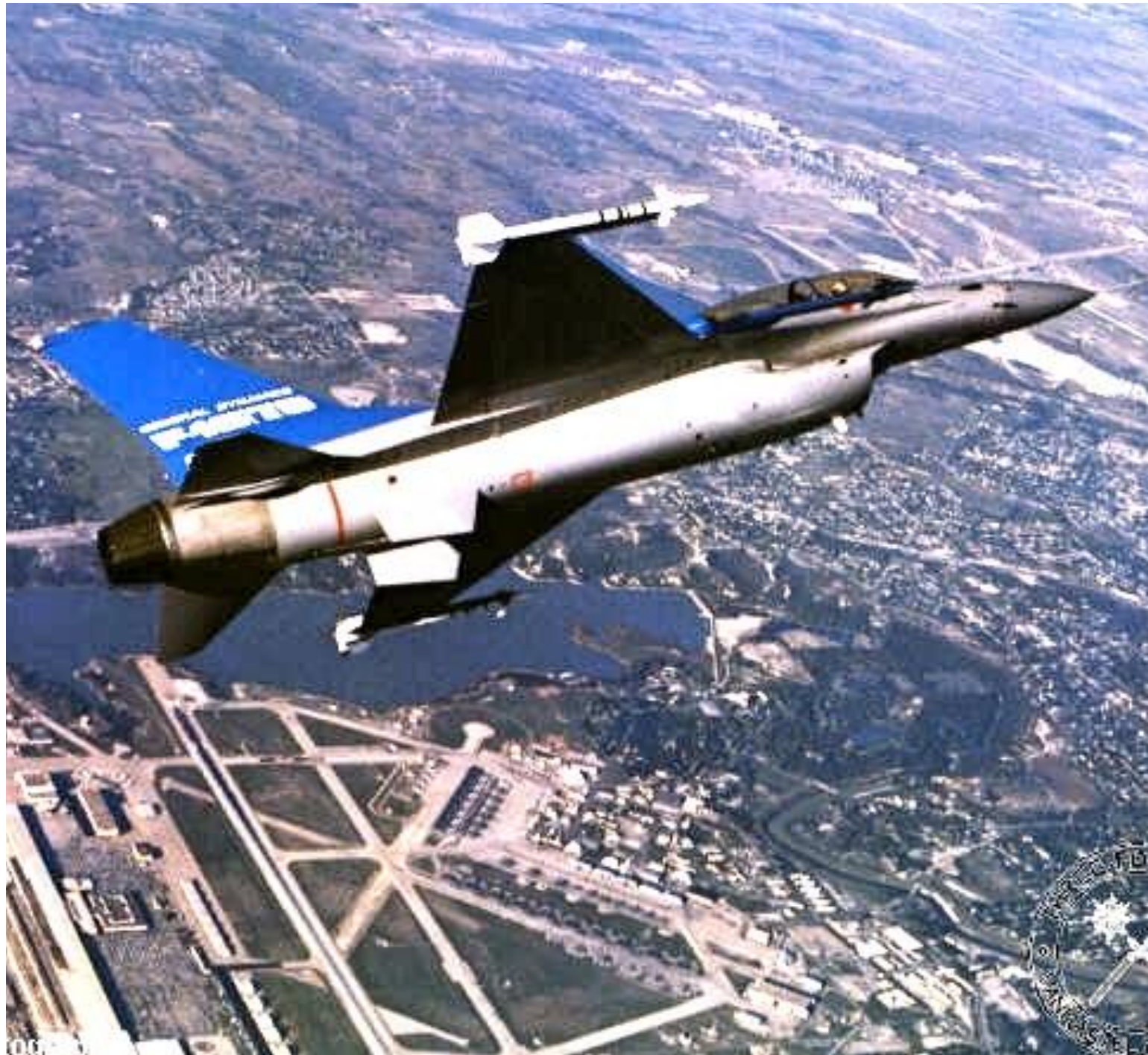
This FSD F-16D is shown over the General Dynamics factory at JRB Fort Worth after being fit with a J79-GE-119 to demonstrate a “low end” Viper for export markets, a result of President Carter’s ill-fated attempt to limit the spread of high tech weapons; the stretched fuselage is very obvious. (USAF photo via F16.net)
