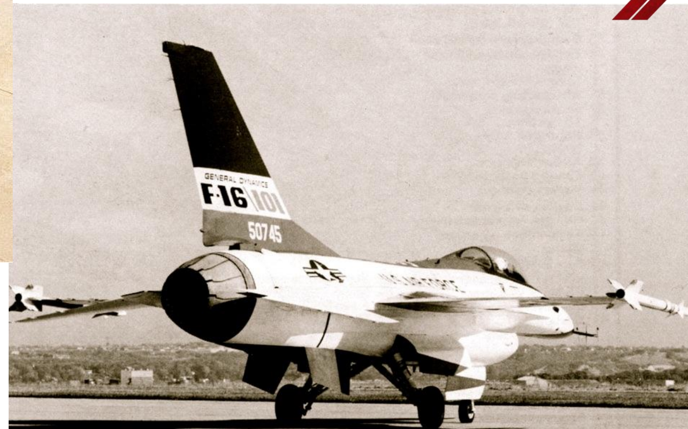
The very first Full Scale Development F-16A, 75-0745, was fitted with the test GE F101X engine; it first flew 19 December 1980. (GD photo via f16.net).
